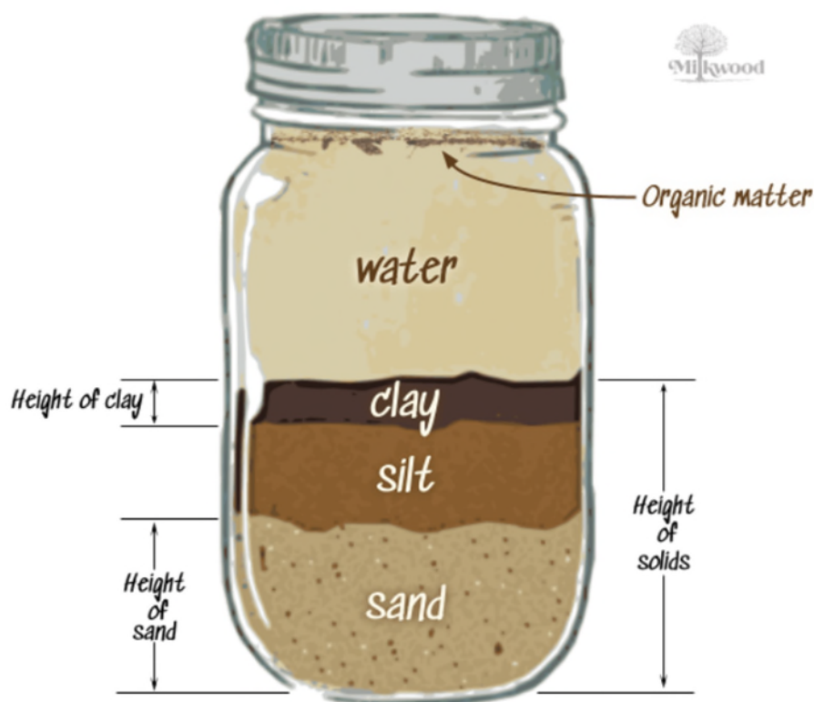
Figure 4-6. Water Jar Test (Milkwood Soil Type Calculator, 2024)
