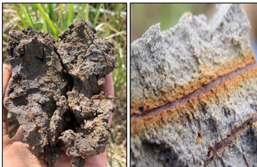
Figure 4-10. Redox Concentrations (Mottling & Oxidized Rhizospheres)
